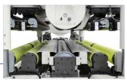
Lower work table with Vulkollan large-sized rollers diameter (210 mm), with independent drives managed by HMI to grant identical speed for each roller.
