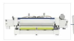
The **unit** is also available in a **"piggyback"** version, a solution designed **to reduce machine footprint** as it can be integrated to a roller and/or pad unit.
