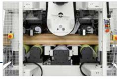
Wide opening of the work table for machining walls up to 500 mm thickness.
