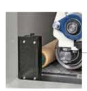
The out-feed pressure roller allows a uniform and intense pressure in calibrating with high removal and sanding of short and narrow pieces
