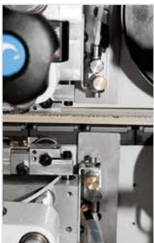
Glue scraping unit with automatic adjustment for machining panel with protective film with different thickness.
