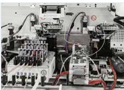
No more machine downtime for glue colour or type change thanks to the "glue switch" system.
