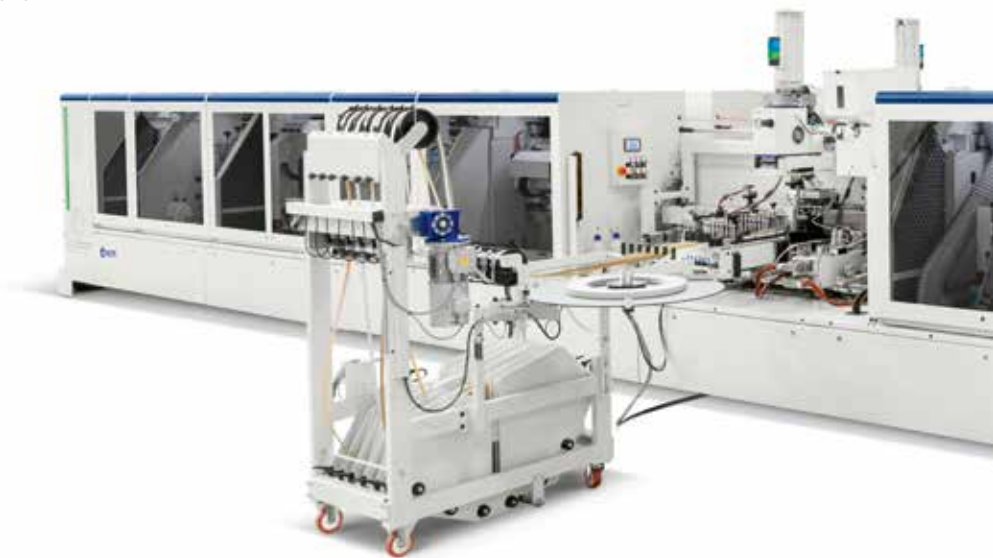
Complete and automatic machining up to 3 radii and infinite thin edges.
