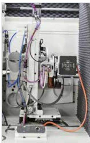
New grooving unit with an increased distance between the groove and the panel side. Proprietary system for an accurate cleaning of the groove.
