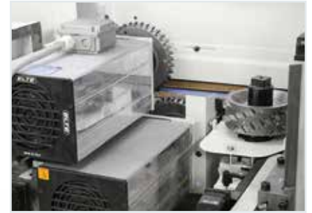
Double hogging unit and compact anti-chipping unit for high working precision.
