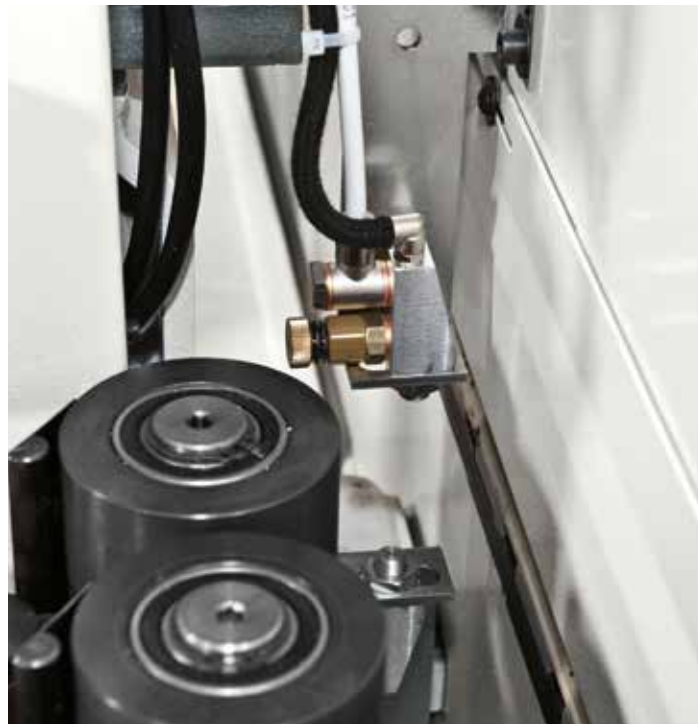
Liquid to cool the temperature of the glue in the area exceeding the edge, in order to keep the tools clean for the subsequent processing (opt.).
