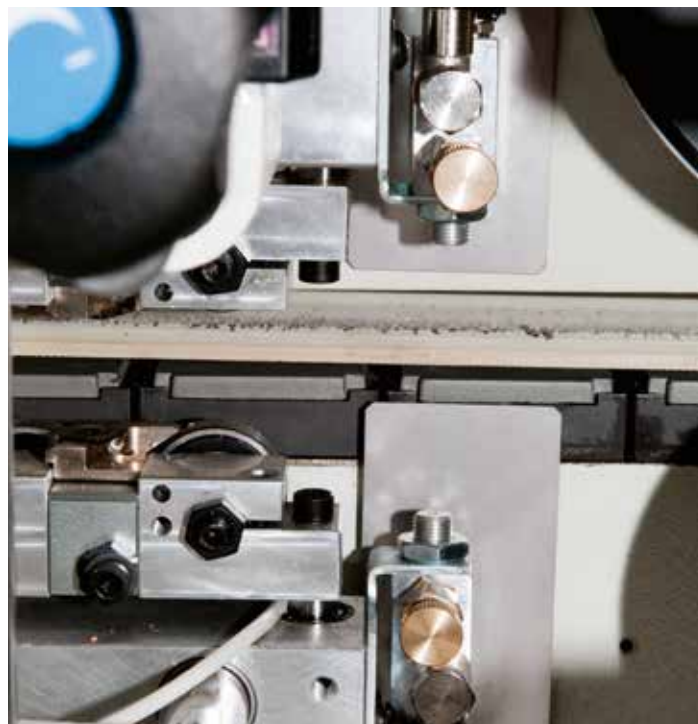
Liquid for smoothing the plastic edge and for brightening the ABS edge (opt.).
