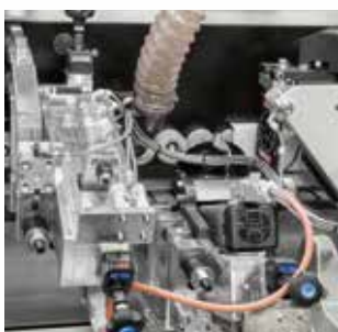
SR-V Trimming-Chamfering unit Machining of two radii, thin edge and solid wood lipping with automatic unit setup.
