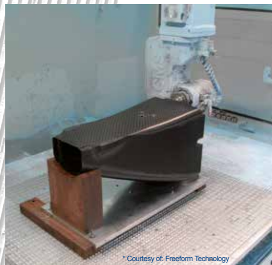
CMS Ares machining centre producing the model and trimming the composite nose component of a competition car
