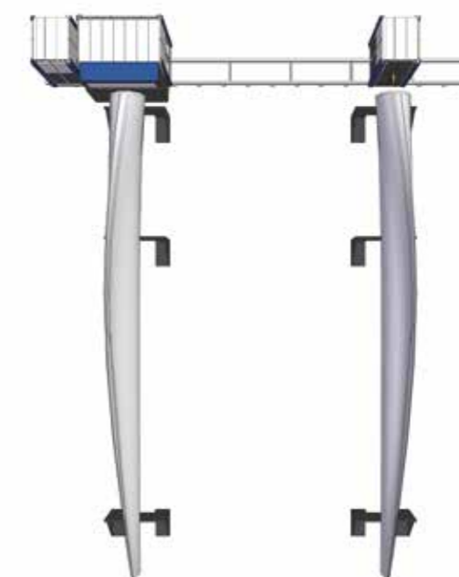
single or double operating unit drilling / milling / T-bolts insertion tandem cycle
