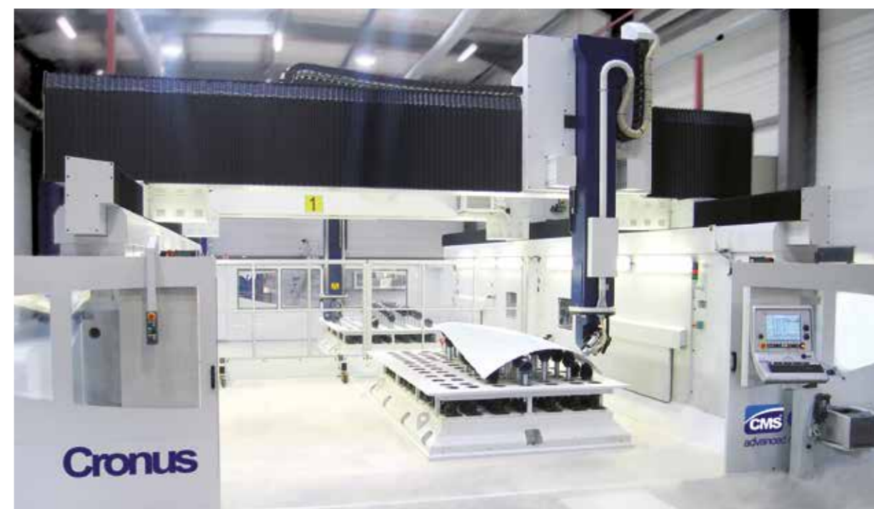
CMS Cronus machining an aircraft part
