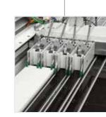
Floating collets: guarantee of excellent results The special shape of the collets allows the safe gripping of plastic sheets and panels, at maximum speed and with perfect parallelism even on surfaces that are not perfectly flat.
