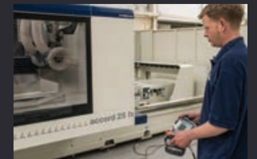
SCM Tecpad mobile console to keep a close check on machining operations
