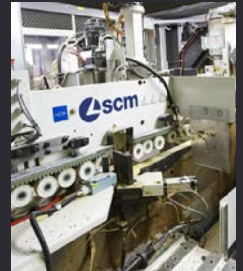
Routing and drilling centre Fleximat in the System 8C line integrated
