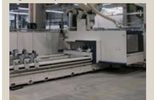
CNC machining centre Accord 40 FX for the HF410 window system
