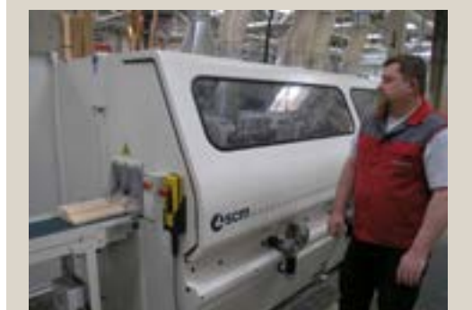
Automatic throughfeed moulders Topset XL integrated in the System 8 line
