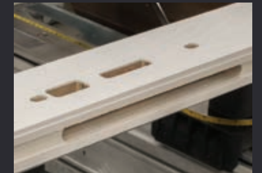
Horizontal routing unit machines door edges for hinge seats and locks.
