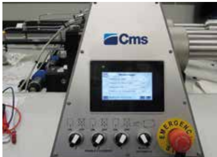
Software-based electronic control of cutting pressure
