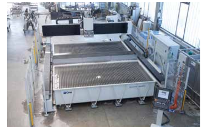
Double tank solution for pendular working (opt)
