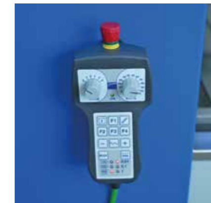
Remote pushbutton pad to control up to 6 axes that allow you to operate close to the cutting surface and set multi-origins
