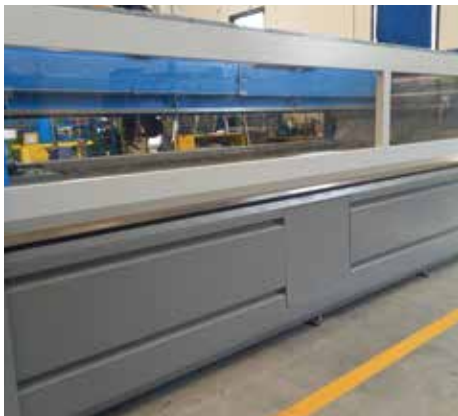
Front and rear hatch with pneumatic movement to better protect the cutting area and reduce the dispersion of water and abrasive material.
