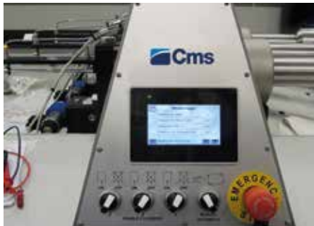
Software-based electronic control of cutting pressure
