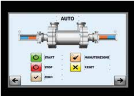
TOUCH CONTROL 17" for remote diagnostics, power check, cycle numbers and pressure electronic management (only on Tecnocut Greenjet Evo stand alone version)
