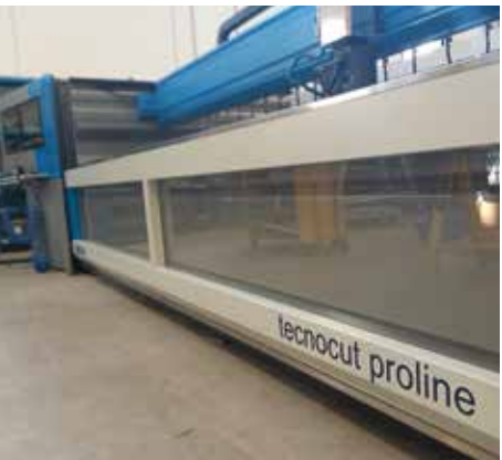
Front and rear hatch with pneumatic movement to better protect the cutting area and reduce the dispersion of water and abrasive material.
