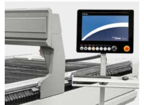
Console on a mobile trolley with standard 21.5" touch screen.
