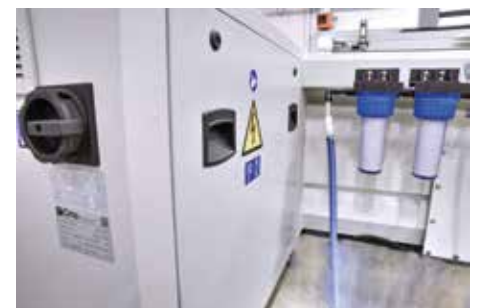
Control panel integrated into the base of the tank to reduce bulk on the ground.
