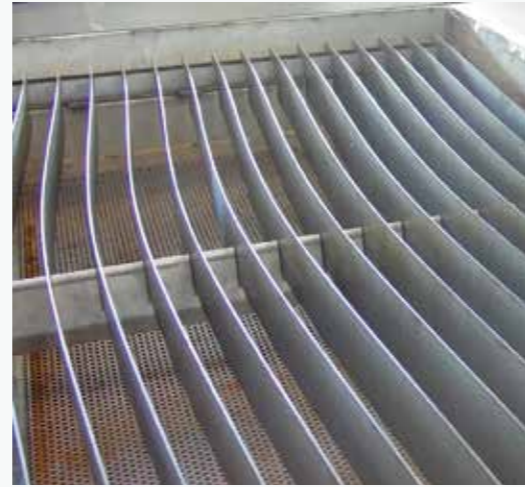
Anti-reverberation table with sheet metal plates available in 35 or 70 mm (optional)
