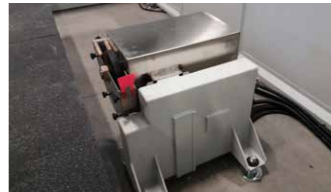
Unit for lower part cut to engrave the lower side of the slab; it allows to insert countertops supports. It can be equipped with drilling unit to realize holes to fix kitchen/ bath countertops. The operations are managed automatically by the machine and need the use of the vacuum manipulator.
