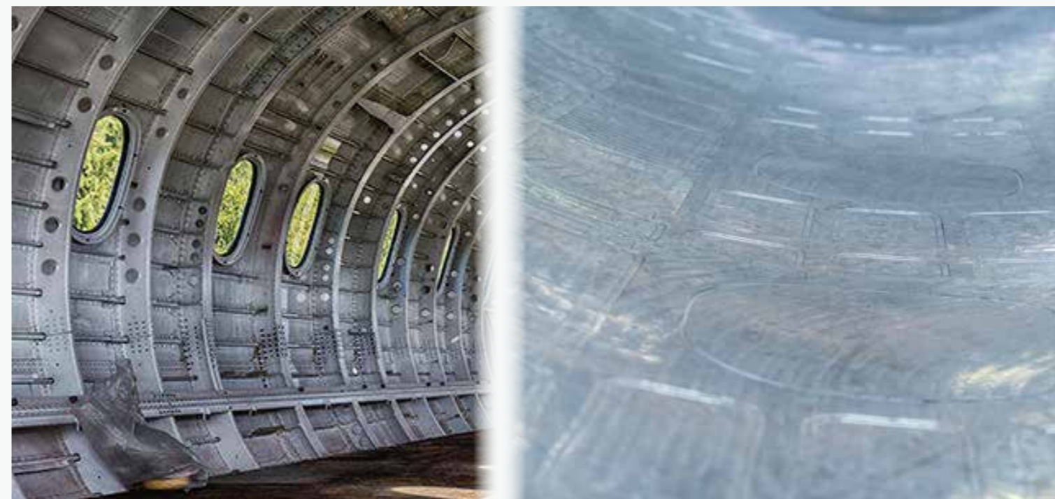
Surface milling of aluminum skins
