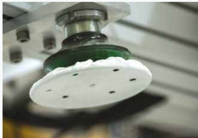
Suction cups for low-e glass sheet management
